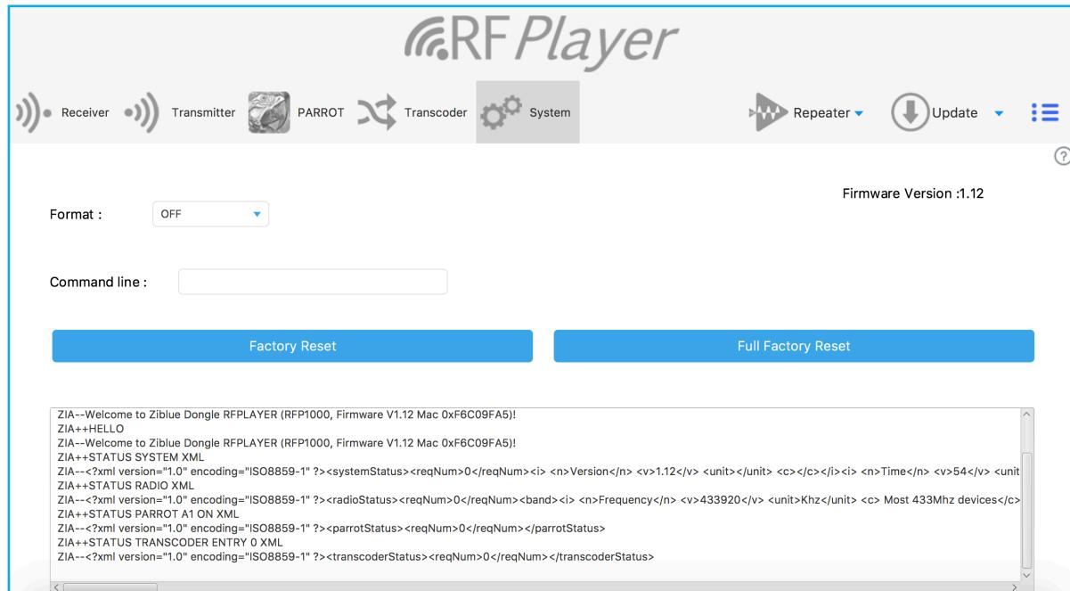
The format of the received RF frames sent to USB port can be specified here. The received frames can be read in the log window below. This function is useful for the developers of RFPLAYER drivers. Note: The Repeater function is enabled only if «Format» is set to OFF.
